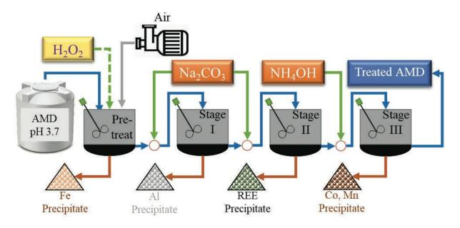
Figure 3. Penn State Process to treat AMD to extract critical minerals
